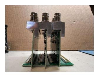
3. Now install the assembly into the FS740 so the BNC connectors on the option card(s) fit through the holes in the back of the instrument. Once the assembly is in place, seat the multi-pin connector into the mating connector on the motherboard of the FS740.
