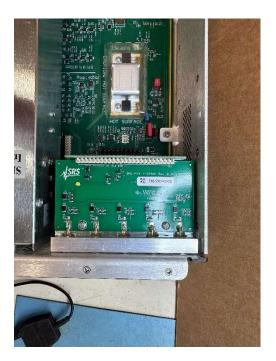
4. Lastly, secure the assembly with the screws provided (see picture below).
